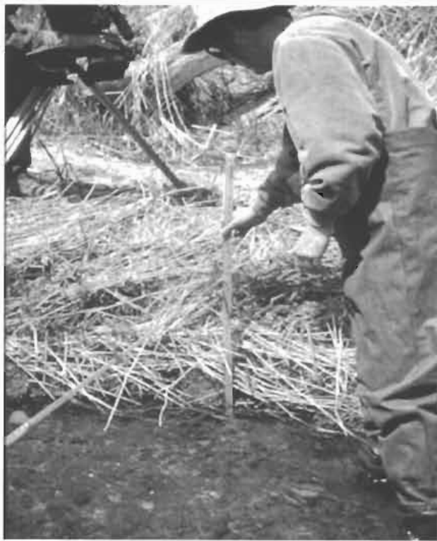
Figure 6: Measuring Height from Channel Bottom to Tape at the Active Channel Boundary.
